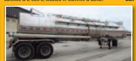
UNIT 10317 – 1995 KROHNERT 6700 USG, MC-307 stainless insulated one compt, all stainless rings and sub-frame, spring ride, safetied.
