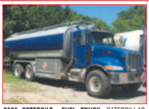
2006 PETERBILT FUEL TRUCK, CATERPILLAR ENGINE; 10 SPD TRANSMISSION; 20,000 LITER, BOTTOM LOAD, DUAL PUMPING, MIDCOM COMPUTER. 445,000 KMS. -188893
