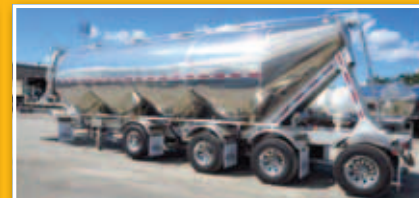
UNIT S403 – NEW 2017 TREMCAR 1850 cu.ft. aluminum pneumatic 6" valves, 5" discharge line, Michelin tires, well spec'd. Call
