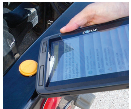
KEEPING TABS: Detroit Connect, which includes Virtual Technician, uses factory-installed telematics tools. A key part is this on-board tablet, developed with Zonar, seen here reading an RFID tag in a driver's pre-trip inspection.
