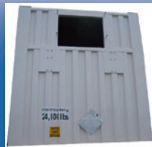
Heated box with front wall prepped for heater.
