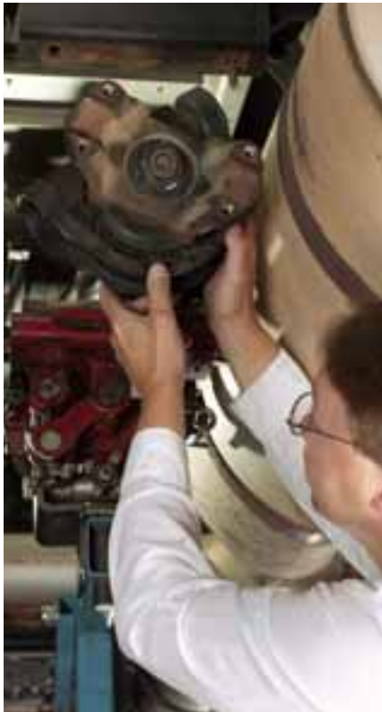
Get your gearing wrong—or under-spec U-joints and driveshaft with a direct-drive transmission—and you could see too many bills for driveline maintenance.
