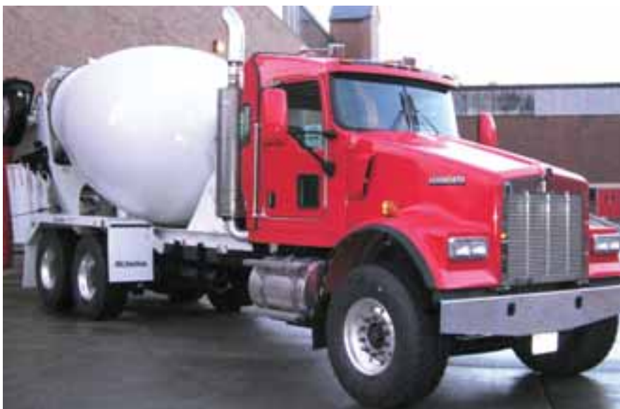
Heavy-duty specialty chassis include tandem and tri-axle drive options up to 69,000-lb, and front ends up to 20,000 lb; engines up to 600 hp, and several DPF placement options depending of PTO requirements.
