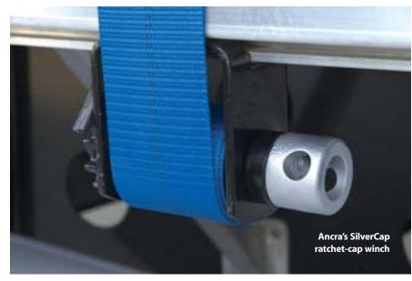
assembly. To secure the load, the cap is simply rotated freely in the opposite direction to position it for the next action to crank down and tighten the load. The winch cap is permanently lubricated and the internal mechanism is protected from dirt and grime. A powder-coated silver-coloured surface adds to the durability of the ratchet-cap winch.
