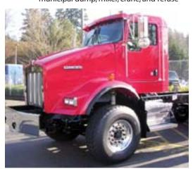
packer configurations. To add the FEPTO option, Kenworth engineers started with the T800 short-hood chassis and designed a straight-through front frame extension. A unique 950-sq-in radiator and stationary grille complete the package.
