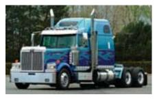
dropped the suspension 2.5 in for applications like boat hauling, plus it gives the truck an *uber*cool look. Ditto for the rear suspension: Western Star's new Low Ride rear suspension now rides at six inches, with the same support as the original AirLiner. Together the new front and rear
