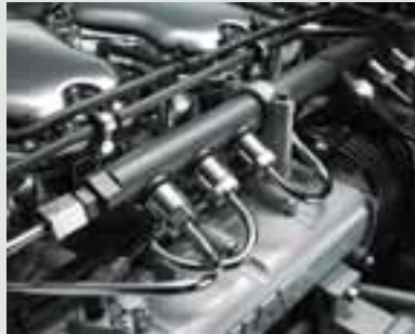
FROM ACROSS THE POND: The XPI high-pressure, common-rail fuel system to be used on 2010 Cummins engines is seen here on Scania's new 13-liter Euro 5 engine, available in European and world markets now.
