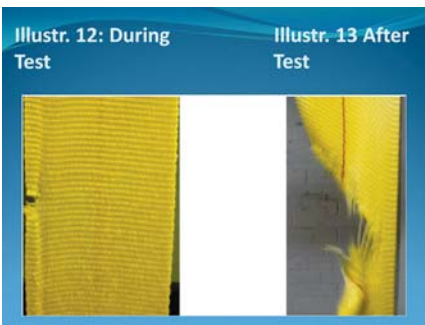
▲ BEHIND THE BELTWAY: Edge cuts and surface abrasion are proving to be harder on straps than originally thought
