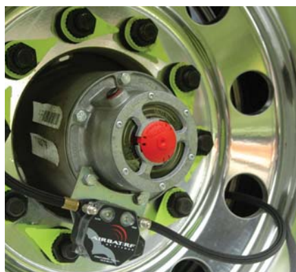
▲ IN THE LOOP: A warning light for the driver and short-range RF data transmission keep everyone in up to speed.
