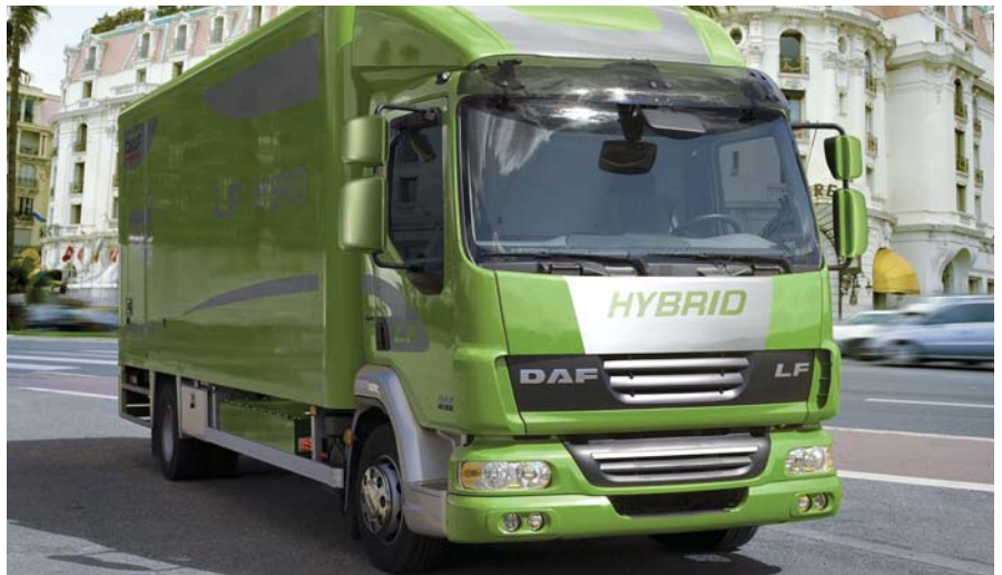
HYBRID DEBUT: DAF's LF45 hybrid truck will enter production at the end of this year. It uses Eaton's hybrid powertrain with a 6-speed Autoshift gearbox.
