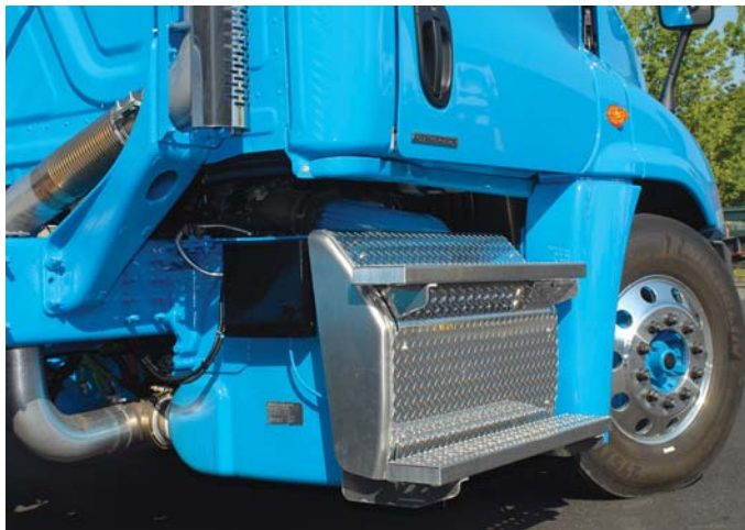
▲ PRACTICAL MATTERS: The Blue-Tec 1-Box aftertreatment system fits neatly beneath the passenger door. The black box contains the dosing meter. The hose on the right leads to the injector nozzle.
