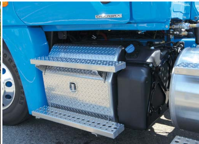
▲ FUEL-PROOF: DEF tanks come in three sizes, mated to the vehicle's fuel capacity (13 gallon shown). The filler necks are sonically welded and are sized to prevent the insertion of diesel nozzles.
