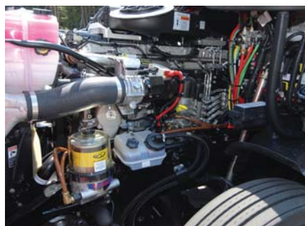
EXHAUSTIVE MAKEOVER: Detroit Diesel's DD15 in EPA 2010 dress. It looks the same as the '07 version because all the new stuff is downstream of the turbocharger.
