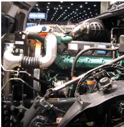
PASSIVE RESISTANCE: Like its Mack stablemates, this 2010 Volvo D13 won't do active DPF regens.
