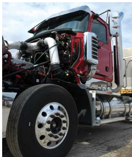
AIR SUPREMACY: Twin polished-metal air intakes minimize moisture and prevents debris from reaching the filter elements. Air intake piping is smooth and non-restrictive promoting high-volume airflow.
