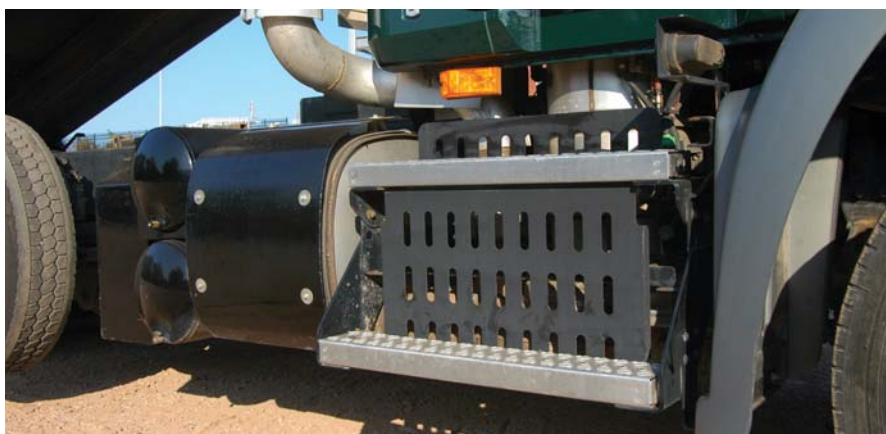
▲ NOW YOU SCR IT, NOW YOU DON'T: Mack places the DPF under the passenger door, behind the metal grate in the photo. The DEF injector is near the outlet of the DPF. The black box-like piece in front of the air tanks is the prototype SCR catalyst container/muffler.
