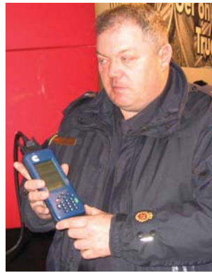
Former OPP Sgt. Cam Woolley demonstrates how speed limiter data is extracted from a truck engine's ECM.
