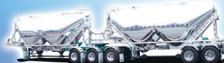
Tremcar Dry Bulk Pneumatic B-Train, 1100 cu. ft. each unit Intraax Suspension, Aluminum Wheels
