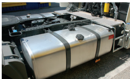
At LKW Augustin in Austria, fuel economy has increased by as much as 10 percent in the fleet's 700 MAN and Mercedes trucks running SCR. Photo above shows a combined diesel/urea tank on an MAN tractor—1,300 liters of fuel in one side, 85 of urea in the other.
